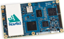
OEM628 Size: 60 x 100 x 9.1 mm Weight: 37 g
